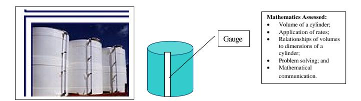
You have been hired by the Number One Tank Gauge Company to provide them with scales to attach to the tanks they sell for holding water. The scales will be transparent glass tubes in which the water in the tube will be at the same level as the water in the tank.
